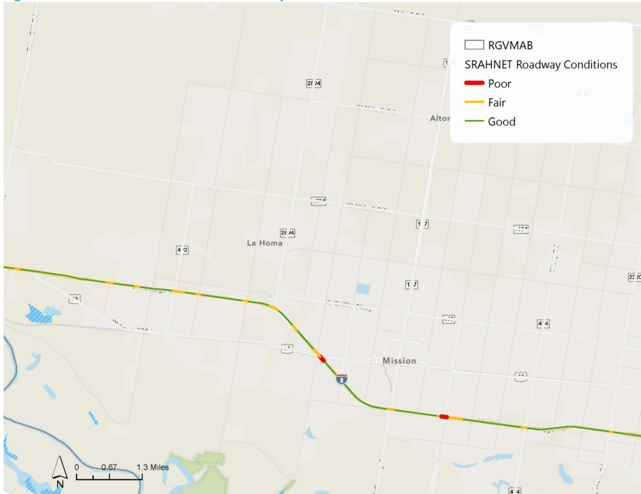
Figure 14 displays Mission area NHS STRAHNET roadway pavement conditions. Two small segments on IH 2 have a poor rating condition on the southside of the BUS 83 overpass and the west side of the FM 396 overpass.
