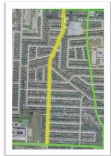
Figure 3-3: Example of Urban Minor Arterial
